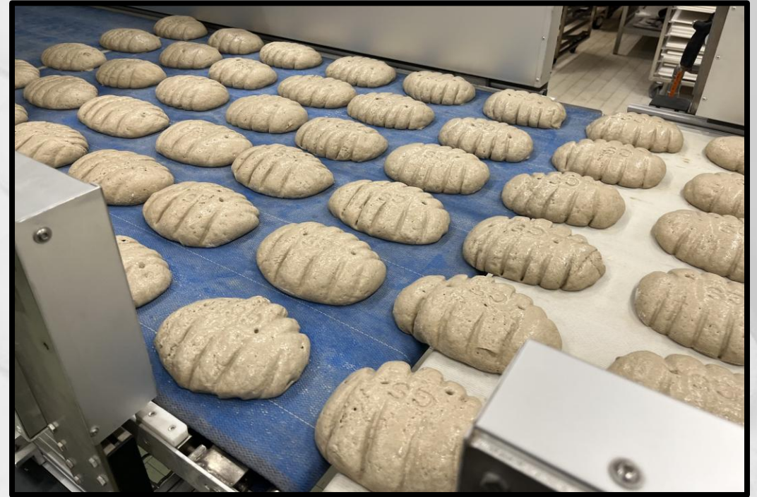
Handover from Crawling Table to Bakelift Pro SideMotion
