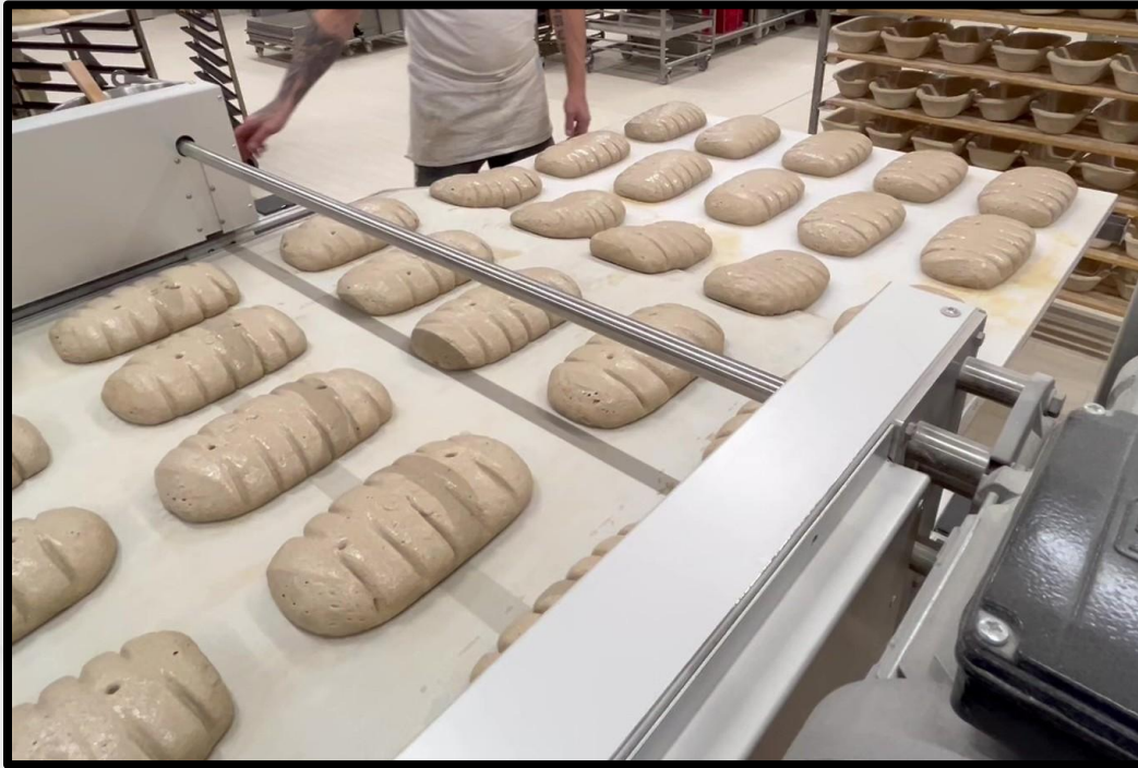
Crawling Table: Dough pieces are crawled from peelboards
